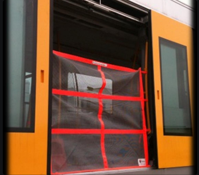
DEPOT SAFETY NET INSTALLED IN A CARRIAGE DOORWAY
