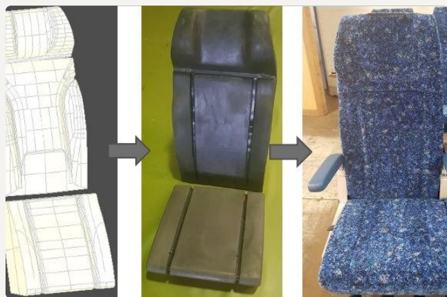
3D MODEL → MOULDED FOAM → TRIMMED SEAT
