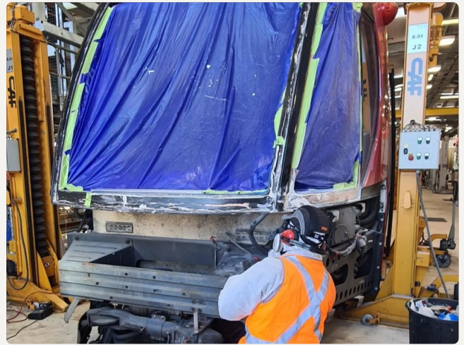
GRP COLLISION REPAIR IN PROGRESS
